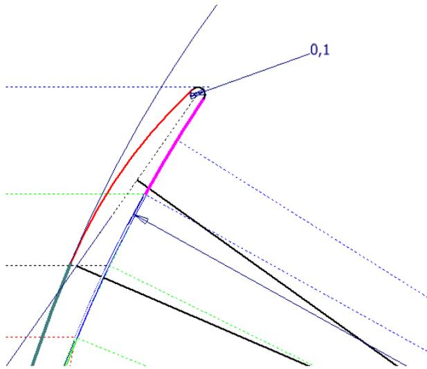
**Fig. 3** The closing arc of 0.1 mm diameter and the smoothing arc (red color)
