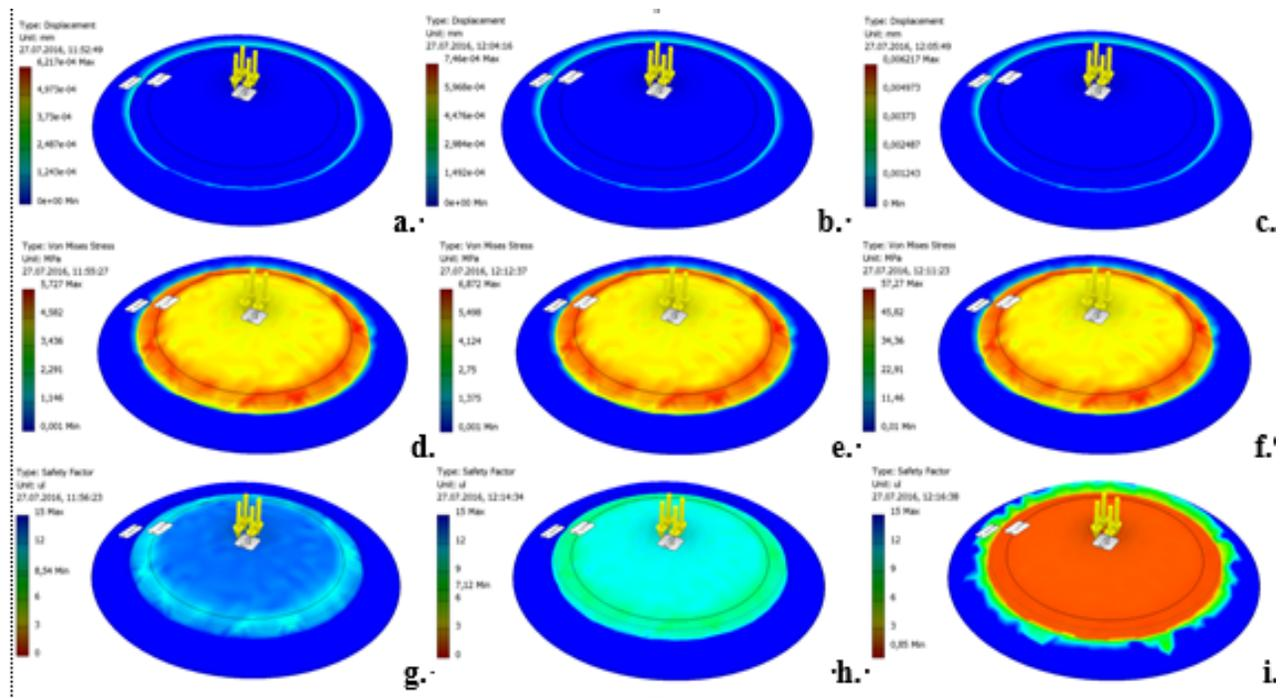
**Fig. 6** Finite element analysis for PMMA: displacement magnitude of the contact lens (for a.10 MPa, b.12 MPa, c.100 MPa), Von Mises Stress with high values in the compressed area (for d.10 MPa, e.12 MPa, f.100 MPa), and lowest safety factor identified in the compressed area (for g.10 MPa, h.12 MPa, i.100 MPa)
