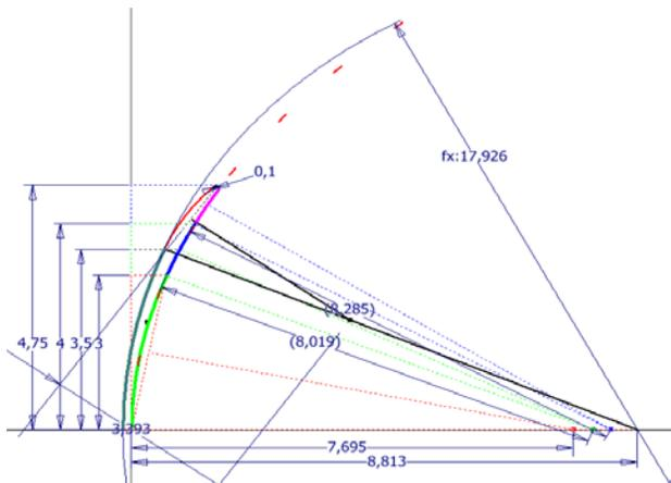
**Fig. 4** The contour used to obtain by revolving the 3D shape of the contact lens
