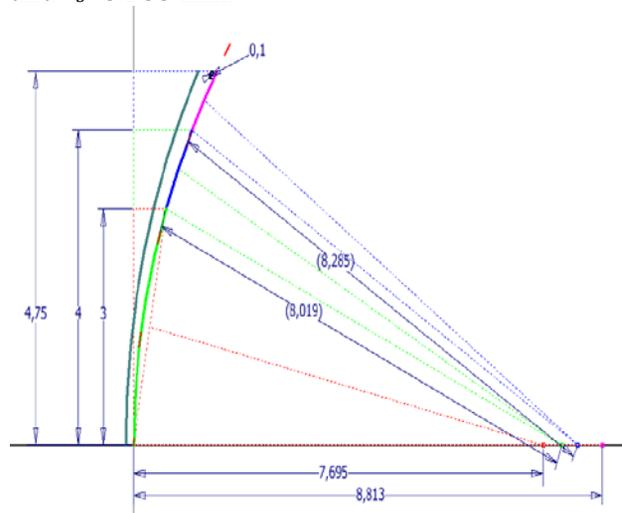
Fig. 2 Back tri-curve line, and the front line of the contact lens (dimensions are in mm)
