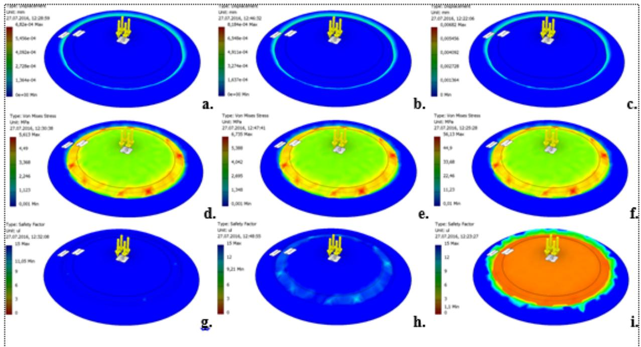
**Fig. 7** Finite element analysis for polycarbonate: displacement magnitude (for **a.**10 MPa, **b.**12 MPa, **c.**100 MPa), Von Mises Stress with high values in the compressed area (for **d.**10 MPa, **e.**12 MPa, **f.**100 MPa), and lowest safety factor identified in the compressed area (for **g.**10 MPa, **h.**12 MPa, **i.**100 MPa)
