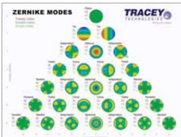
Fig. 2. This figure shows the most common shapes of aberrations when a wavefront of light passes through an eye with imperfect vision. A theoretically perfect eye is represented by an aberration-free flat plane, named piston (top). Wavefront aberrations can be mathematically
